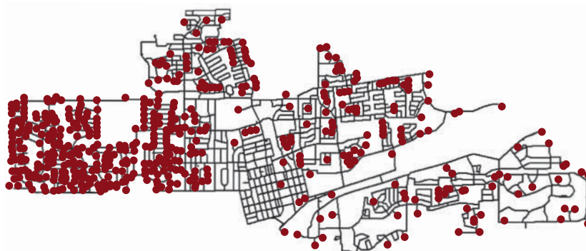
FIGURE 11 The locations of intrusion using the pressure-insensitive demand model
