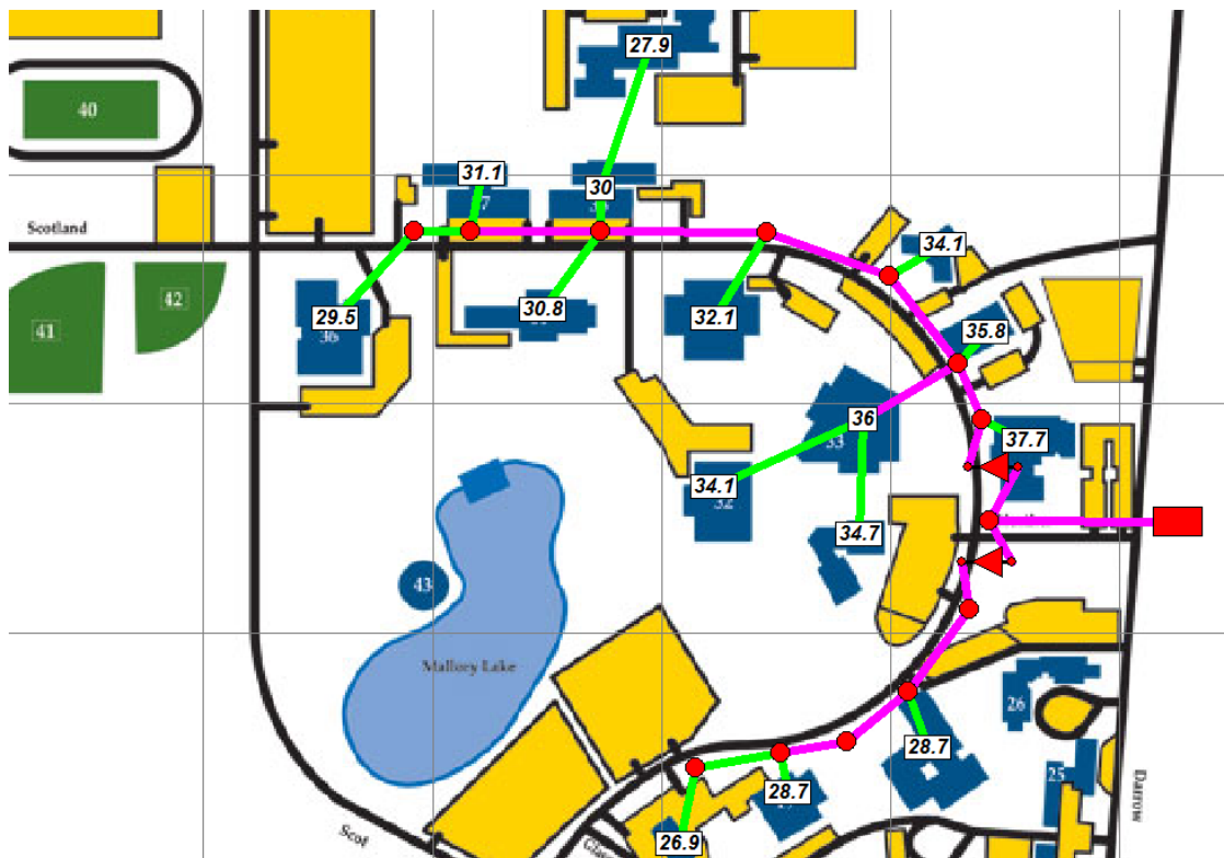
Figure CF-19 Gas Distribution Model Results – Building Pressures
