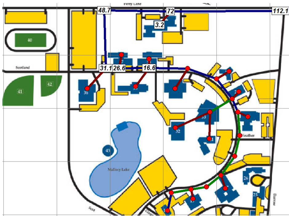
Figure CF-27b Superheated Steam Distribution – Superheat (400 #/hr)
